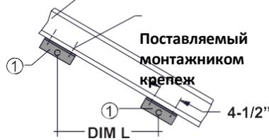
DIM L = Distance between mounting holes. (Refer to owner's manual)
